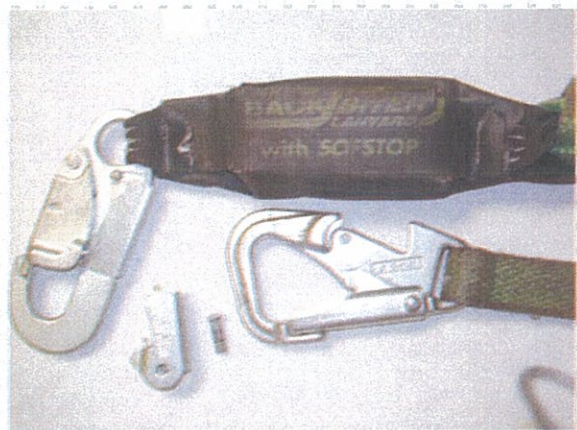
Miller Back Biter lanyard being used by employee at time of failure. Date of manufacturer of this particular lanyard is 05/09/08. In service date of this lanyard was 02/17/09.
